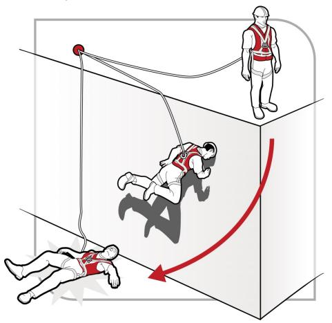
Figure 23 'Swing down': the length of the lanyard and positioning of the anchor allow contact with the ground
