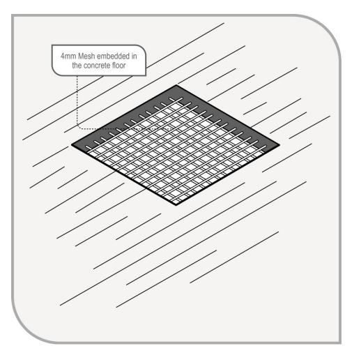
Figure 5 Mesh embedded in a concrete floor
