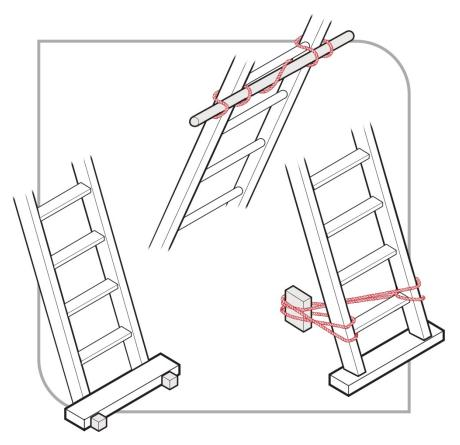
Figure 29 Examples effectively securing a ladder
