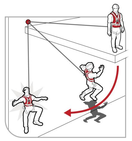
Figure 24 During 'swing back' the length of the lanyard and positioning of the anchor may allow the worker to hit the structure
