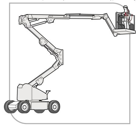
Figure 10 Boom-type elevating work platform
