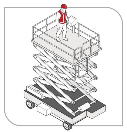
Figure 11 Scissor-lift elevating work platform
