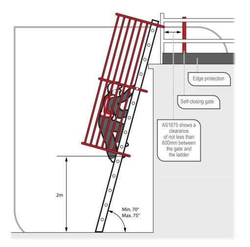
Figure 32 Fixed ladder with ladder cage
