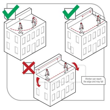
Figure 19 Restraint technique options
