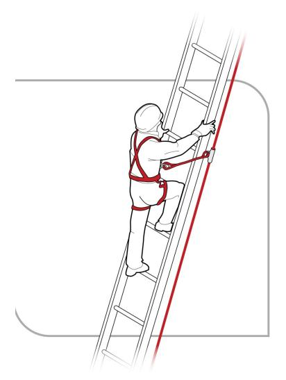
Figure 25 Anchorage line system
