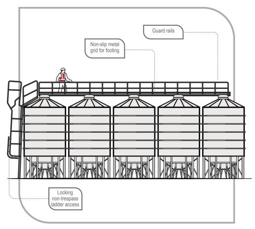
Figure 4 Silos with platform and guard rails
