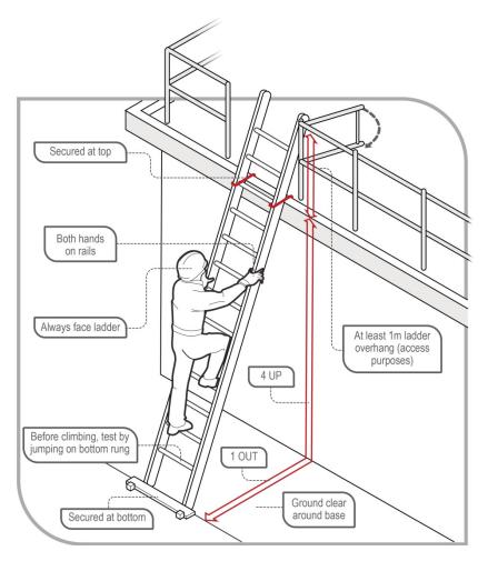
Figure 30 Example of acceptable ladder use
