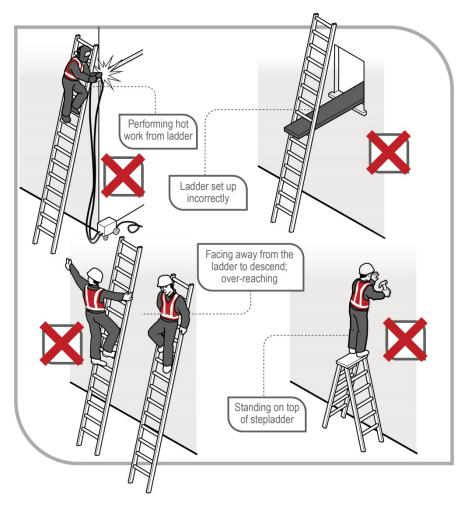
Figure 31 Examples of unsafe ladder use
