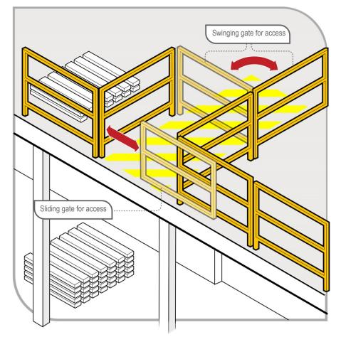
Figure 3 Mezzanine floor barrier
