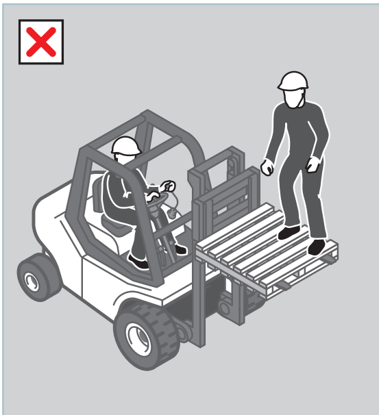
Figure 13 – Using a forklift as a working platform or to gain extra height by standing on the tynes or a pallet is an unacceptable practice.
