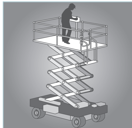
Figure 10 – An example of a scissor-lift elevating work platform.
